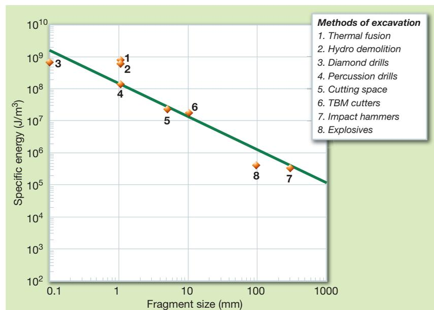
This figure leads to the important conclusion that the SEE is related exponentially to the size of rock fragments produced during the rock breaking process, and that excavation by explosives consumes the least amount of energy among the methods studied. TBM boring falls in the middle of the range.
