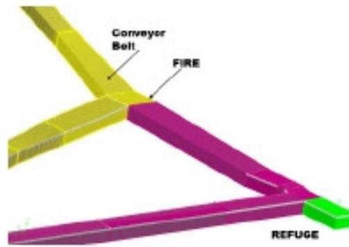
Figure.1: CFD simulation of mine fire, essential features
