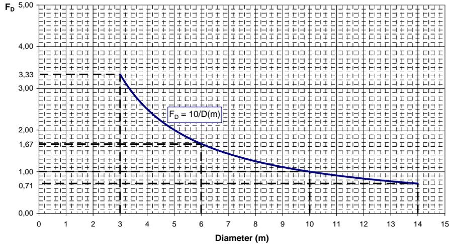
Figure 3. Variation of factor  $F_D$  with tunnel diameter
