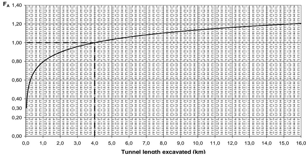
Figure 2. Variation of factor  $F_A$  with the excavated tunnel length
