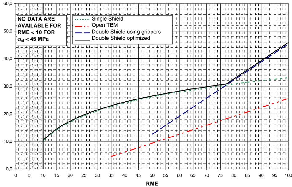
Figure 7b. Correlations between RME and  $ARA_T$  for different types of TBMs in rock masses featuring rock material with  $\sigma_{ci} < 45$  MPa.
