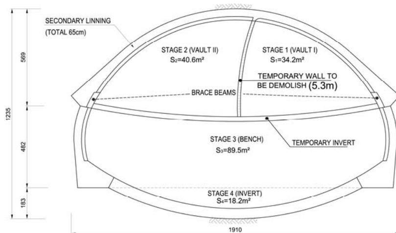
**Figure 4. East Tunnel of Los Leones Station constructed by SSV method.**
