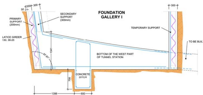
**Figure 7. Bottom ditches' details.**
