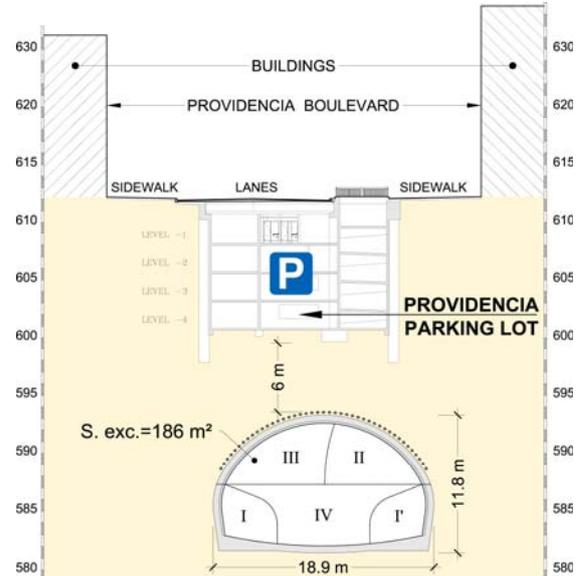
**Figure 3. Cross-section of Los Leones Station.**
