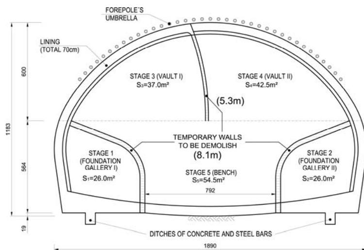
**Figure 6. SFG method at the West part of Los Leones Tunnel Station.**
