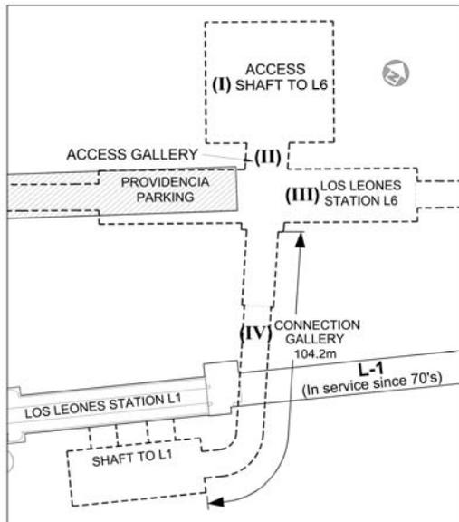
**Figure 2. L-6 Los Leones Station and its connection with L1.**
