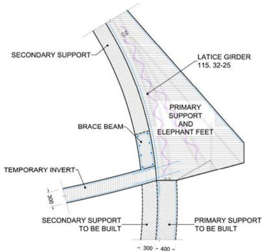
**Figure 5. Elephant foot and brace beams details.**
